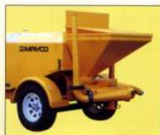
3" x 2" reducer is standard; swings up and away for easy travel and cleaning
