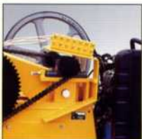
Central lubrication system for quick and easy maintenance.
